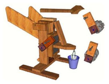
The Easy BioGrind<sub> $\odot$ </sub> biomass grinder was designed to grind dry biomass and to accomplish a number of goals. The objectives were the flexibility to grind a wide variety of dry biomasses, low-cost, easy to build using mostly hand tools, easy to operate, easy to maintain and require no welding.
