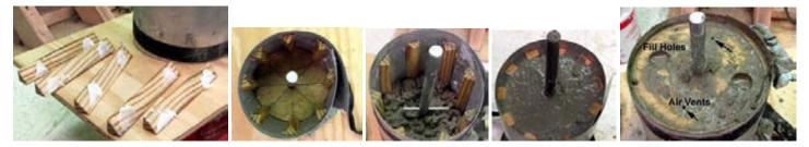
Remove the cylinder when you are comfortable that the concrete has cured sufficiently to be able to wire brush the teeth to expose the aggregate. Do not wire brush the V section of the teeth. Again, keep the end caps in place for about 24 hours until the concrete has cured enough to safely remove them without damaging the edges. Again, cover with a wet cloth and plastic and keep wet for curing.
