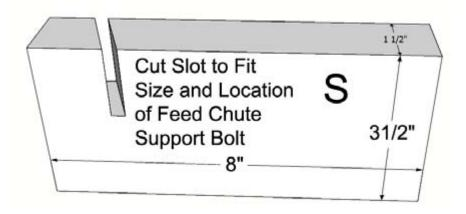
The dimensions are based on a standard lumber size of  $3\frac{1}{2}$  wide X  $1\frac{1}{2}$  thick material, and  $5\frac{1}{2}$  wide X  $1\frac{1}{2}$  thick material. The grinder can be constructed using softwood.
