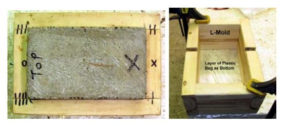
After the no teeth grinding head (NA) has cured for a few days, wrap it tightly in plastic and insert it into the two slots in the L-Mold. Fill the mold with concrete and jiggle to remove air bubbles.
