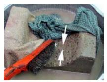
Reassemble the L-Mold and cut the mold into two sections at the cut line. Keep the bottom section of the mold as the holder for the grinding cup.
